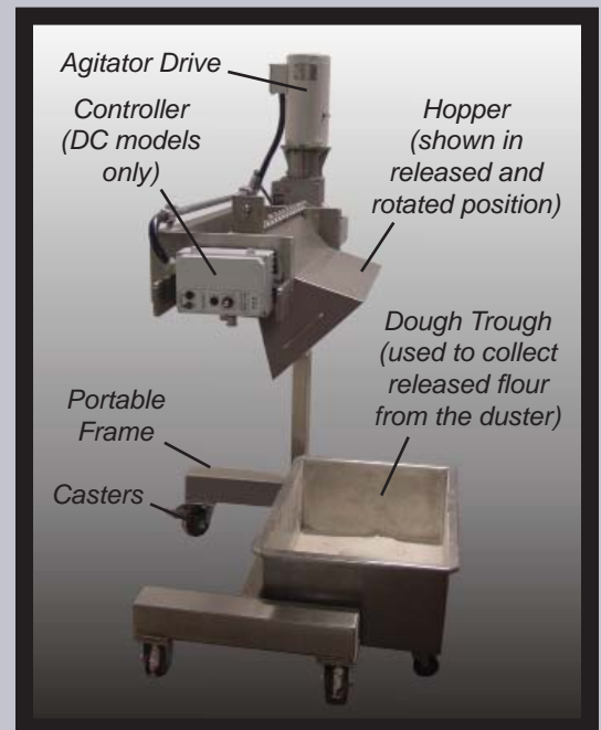
Portable DC Duster/Dispenser (with Quick Release Hopper shown in released and rotated position)
